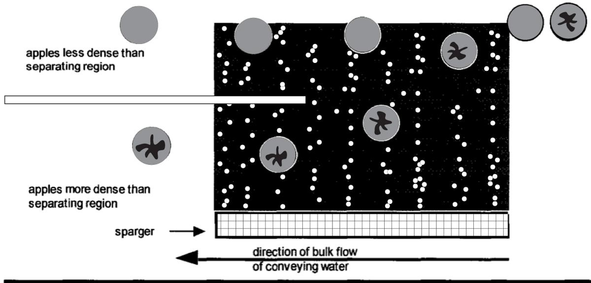
**Figure 5. Schematic depicting the separation of less dense, non-watercore apples (upper stream of fruit - gray spheres) from more dense, watercore-containing fruit (lower fruit stream) (redrawn from Cavalieri et al., 1998).**
